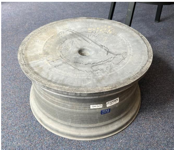
Figure 1: Forged ARW blank
