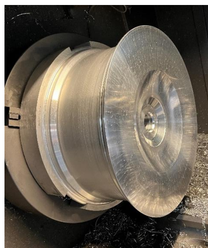
Figure 2: Machined, unfinished ARW
