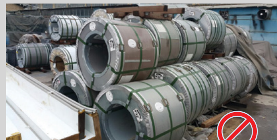
▲ Incorrect outdoor storage (cover not used)
