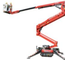
Spider Booms Can fit through doorways and work on soft ground
