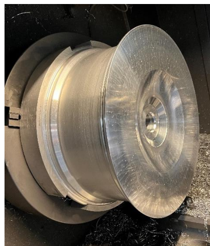
Figure 2: Machined, unfinished ARW
