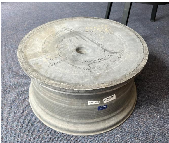
Figure 1: Forged ARW blank
